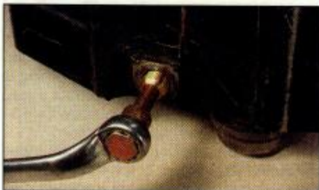
2.22 A thread repair tool being used to correct an internal thread
