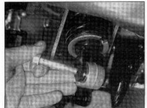
11.2c Remove the shock absorber lower mounting bolt ...
