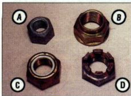
2.4 Plain nut (A), shouldered locknut (B), nylon insert nut (C) and castellated nut (D)
