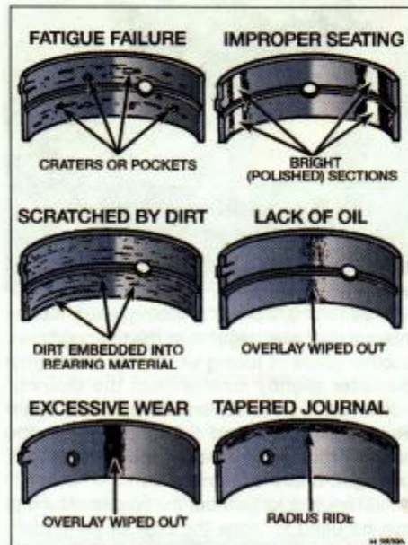
5.17 Typical bearing failures
