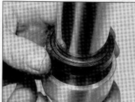
7.22 Make sure the oil seal is the correct way up
