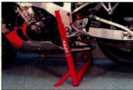
1.3 This auxiliary stand attaches to the swingarm pivot
