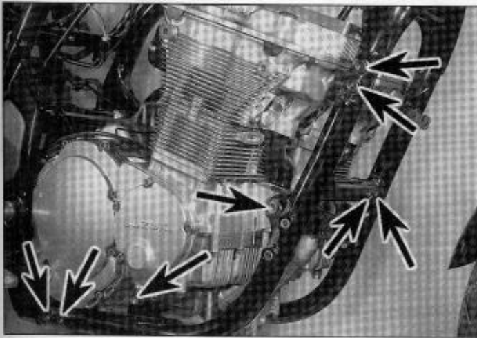
5.19a Remove the bolts (arrows) . . .
