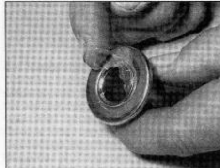
14.10a Smear the spacer contact surfaces with grease (600 model spacer shown)
