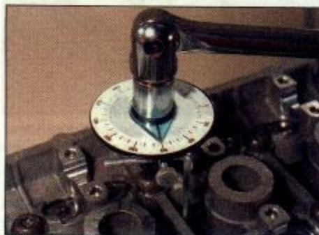
4.2 Angle tightening can be accomplished with a torque-angle gauge ...
