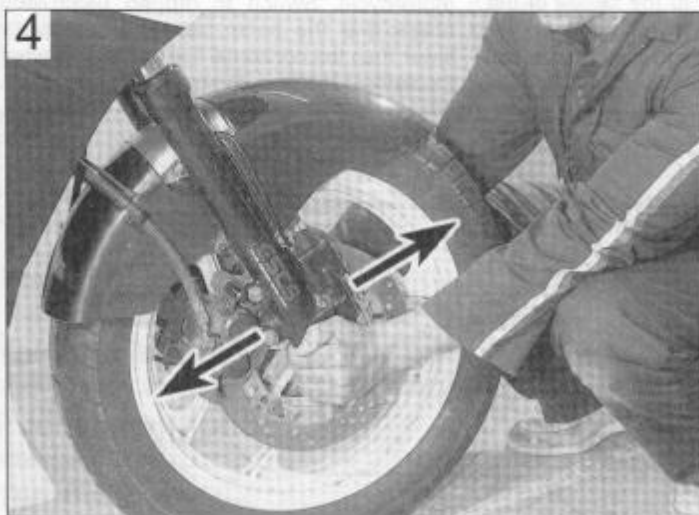
4 Checking the steering head bearings for freeplay
