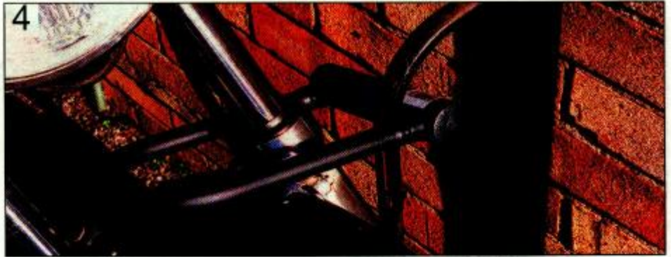
U-locks can be used to secure the bike to a solid object – ensure you purchase one which is long enough
