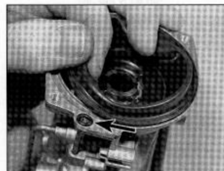
7.16 Carefully separate the diaphragm from the body and lift it and the piston out. Also remove the O-ring (arrow)
