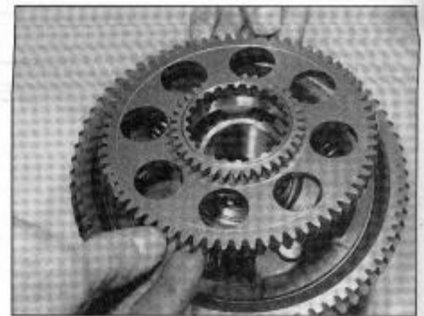
18.9 Lift the alternator/oil pump drive gear off the back of the clutch housing
