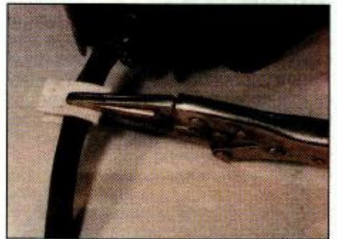
9.4 ... or thick card and self-locking grips
