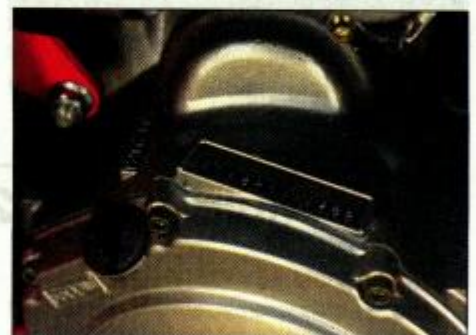
The engine number is stamped into the top of the crankcase behind the cylinder block
