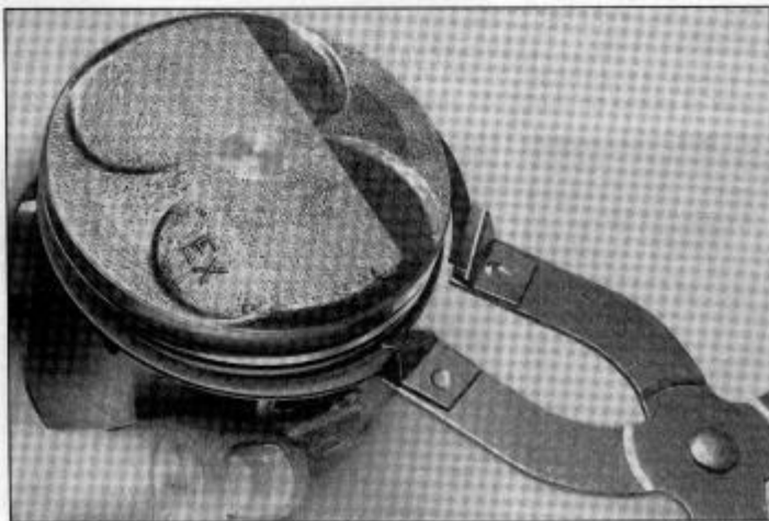
16.5a Removing the piston rings using a ring removal and installation tool
