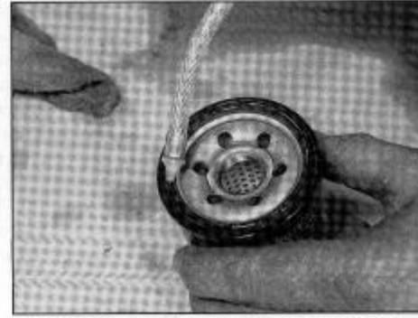
20.3a Smear clean engine oil onto the sealing ring . . .
