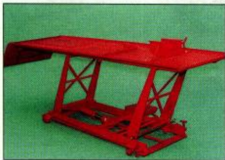
1.1 Hydraulic motorcycle ramp
