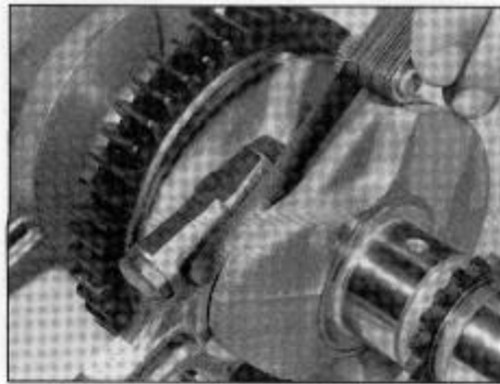
31.2 Slip a feeler gauge between the connecting rod and the crank web to check side clearance
