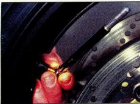
1 Check the tyre pressures when the tyres are cold and keep them properly inflated.
