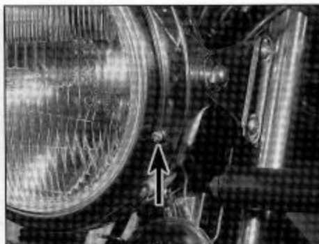
33.2 Headlight beam horizontal adjuster (arrow)
