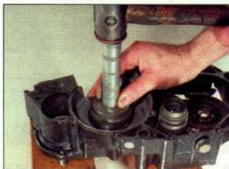
5.1 Using a bearing driver against the bearing's outer race
