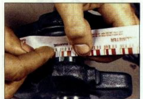
3.16 Measuring the width of the crushed Plastigauge
