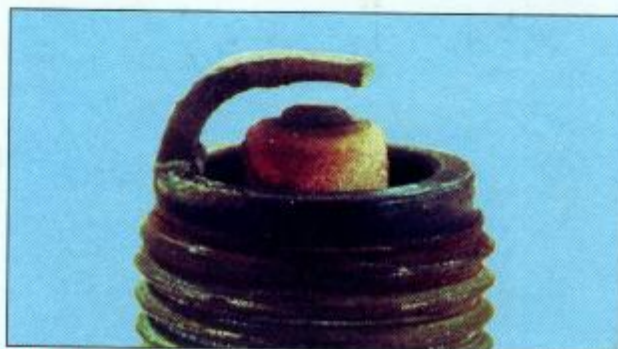
Worn plug – Worn electrodes will cause poor starting in damp or cold conditions and will also waste fuel.
