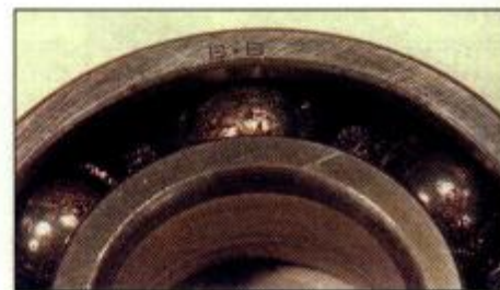
5.18 Example of ball journal bearing with damaged balls and cages
