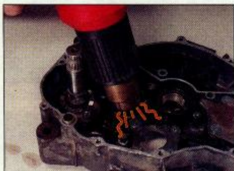
2.15 Using heat to free a seized fastener
