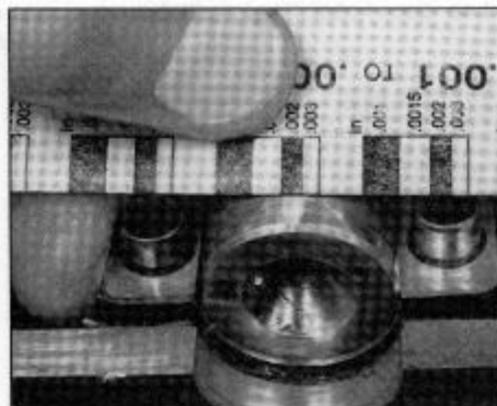
11.16a Compare the width of the crushed Plastigauge to the scale provided with it to obtain the clearance
