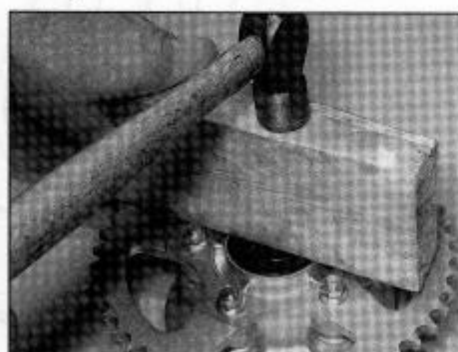
16.30 A piece of wood can be used to drive the bearing seal onto the bearing
