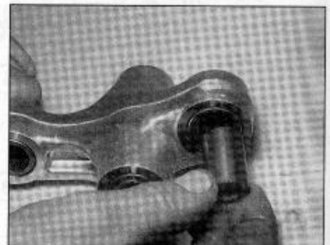
11.10 Lubricate all the bearings with grease and install the spacers
