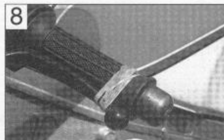
Hold clutch lever back against the handlebar with elastic bands or a cable tie
