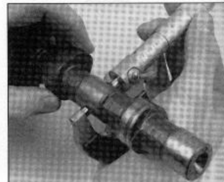
11.16b Measure the cam bearing journal with a micrometer
