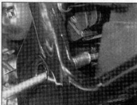
10.4b . . . then unscrew the bolt using a socket extension inserted through the hole . . .
