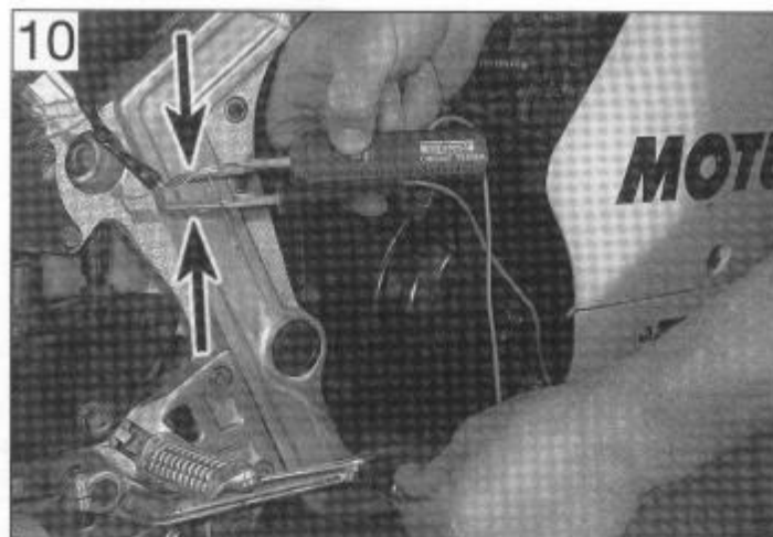
10 Continuity check of rear brake light switch using a continuity tester
