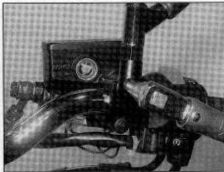
5.21b . . . and tighten the bolts to the specified torque setting
