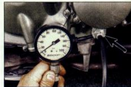
3.21 Oil pressure gauge and take-off point adapter (arrow)
