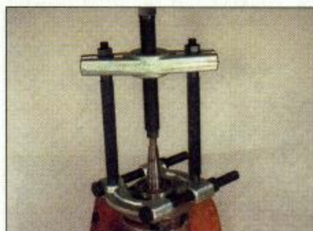
5.3 This bearing puller clamps behind the bearing and pressure is applied to the shaft end to draw the bearing off
