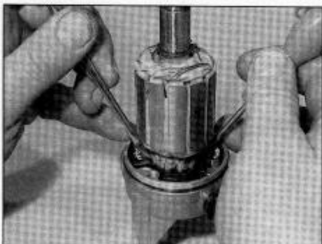
31.15 Hold the brushes back whilst installing the commutator
