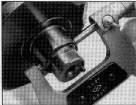
30.24 Measure the diameter of each crankshaft journal
