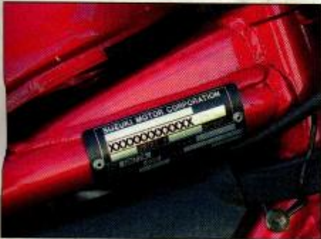
The frame number is stamped on a plate on the right-hand frame spar . . .
