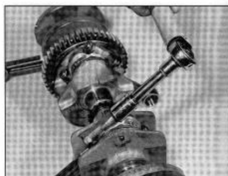
31.23 Tighten the connecting rod cap nuts to the specified torque setting in two stages
