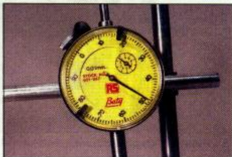
3.17 Dial gauge reading of 1.48 mm
