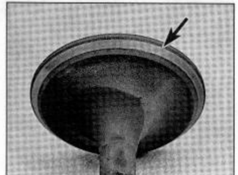
14.24b The face and seat should be the specified width and have a smooth, unbroken appearance (arrow)
