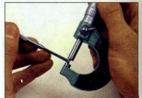
3.10 ... then measure the gauge with a micrometer
