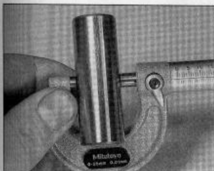
16.13b Measure the external diameter of the pin ...
