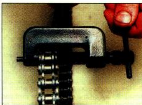
8.1 Tighten the chain breaker to push the pin out of the link ...
