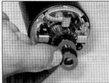
31.24a Install the shims on the rear end of the armature shaft ...
