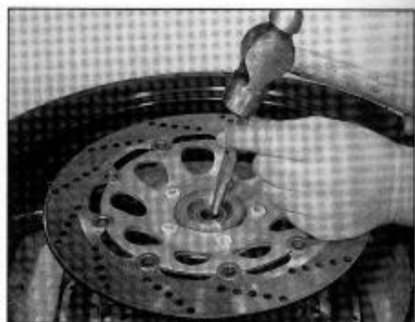
16.3a Using a drift to knock out the bearings
