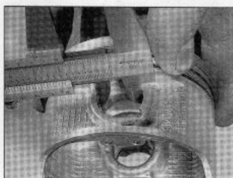
16.13c ... the internal diameter of the bore in the piston ...
