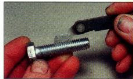
2.12 Using a thread gauge to measure pitch
