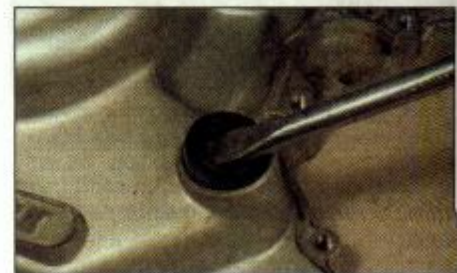
6.1 Prise out oil seals with a large flat-bladed screwdriver
