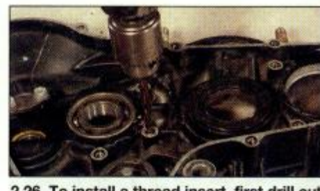
2.26 To install a thread insert, first drill out the original thread ...
