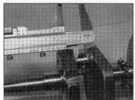
31.7b ... and of the corresponding crankpin
