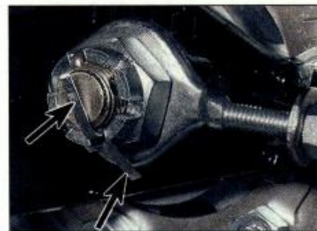
2.5 Bend split pin (cotter pin) arms as shown (arrows) to secure a castellated nut
