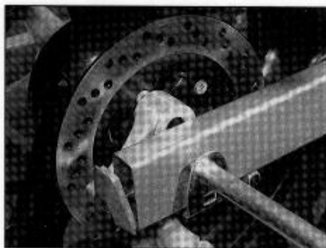
15.11a Install the axle from the right, making sure it passes through all components ...
