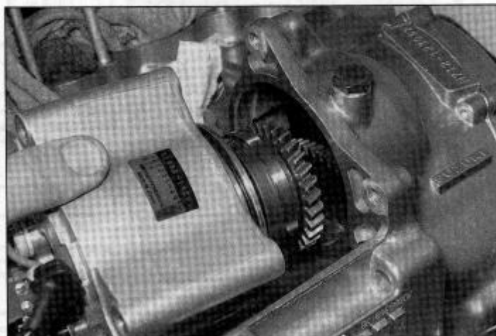
34.18 ... and install the alternator
