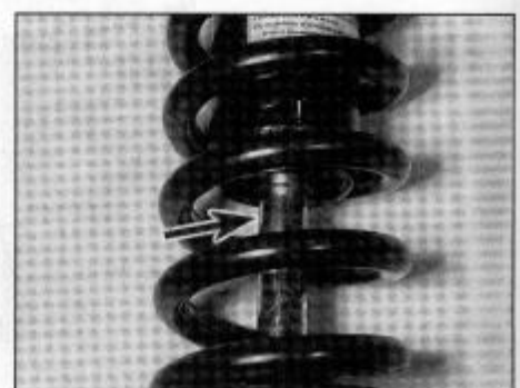
10.6 Inspect the damper rod for pitting and leakage (arrow) . . .
