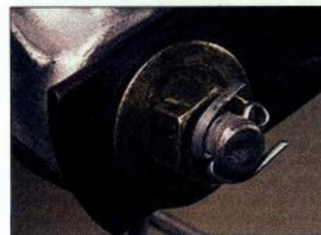
2.6 Bend split pin (cotter pin) arms as shown to secure a plain nut
