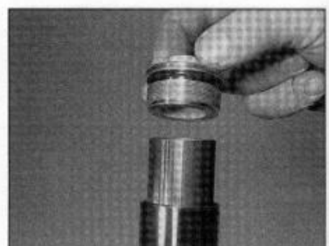
7.27 Fit a new O-ring onto the top bolt and thread the bolt into the fork tube
