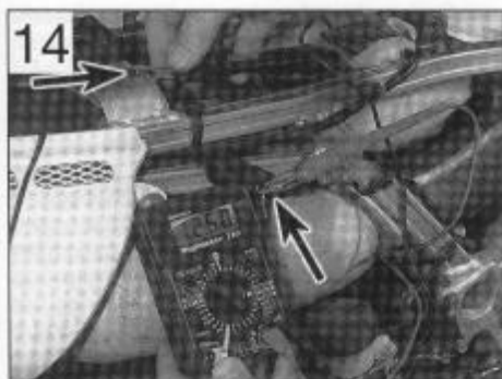
14 Checking for voltage at the rear brake light power supply wire using a meter . . .
