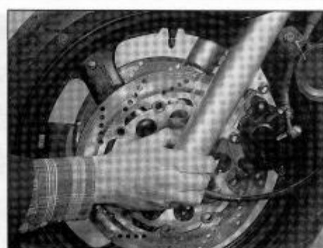
22.4 Checking for play in the steering head bearings
