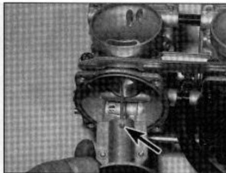
9.11 Install the diaphragm/piston assembly with the indent in the piston (arrow) facing the air intake side
