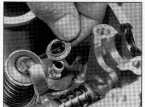
14.28a Install the spring seat
