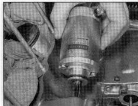
30.7 Fit the starter motor into the crankcase . . .
