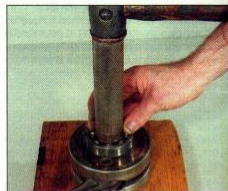
5.5 When installing a bearing on a shaft use a piece of tubing which bears only on the bearing's inner race
