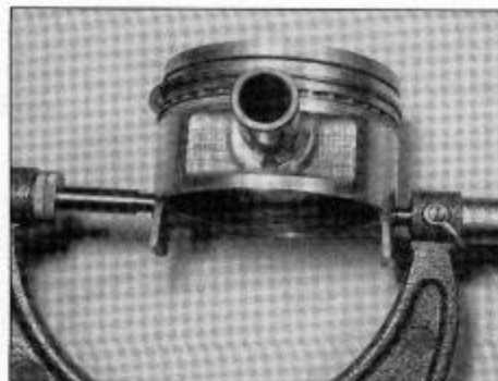
16.12 Measure the piston diameter with a micrometer at the specified distance from the bottom of the skirt
