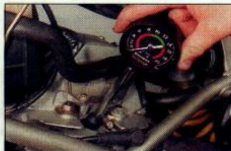
3.20 Using a rubber-cone type cylinder compression gauge
