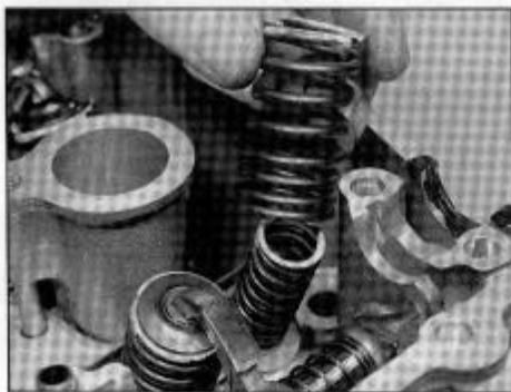
14.29c Install the outer spring with its closer-wound coils at the bottom, next to the head
