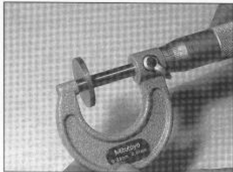
Tappet shims are measured with a micrometer
