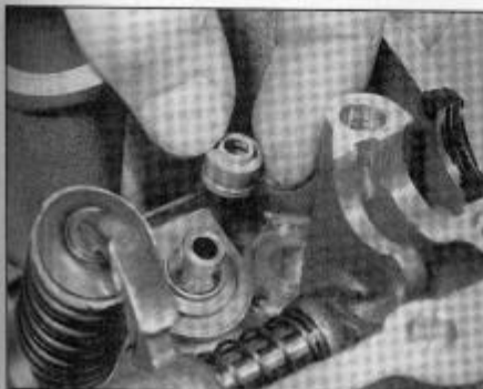
14.28b Fit the oil seal over the valve stem
