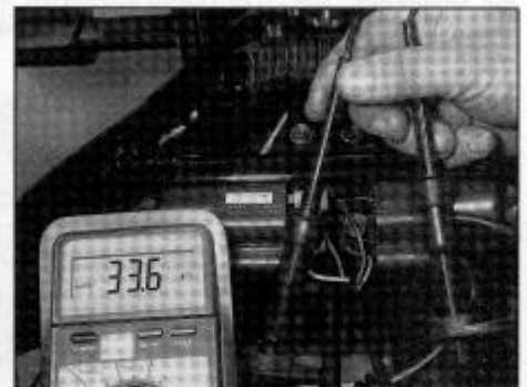
3.6 Ignition coil secondary circuit test connections
