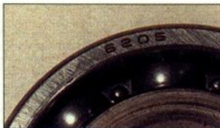
5.16 Typical bearing marking
