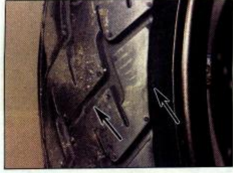
3 Tyre tread wear indicator bar and its location marking (usually either an arrow, a triangle or the letters TWI) on the sidewall (arrows).
