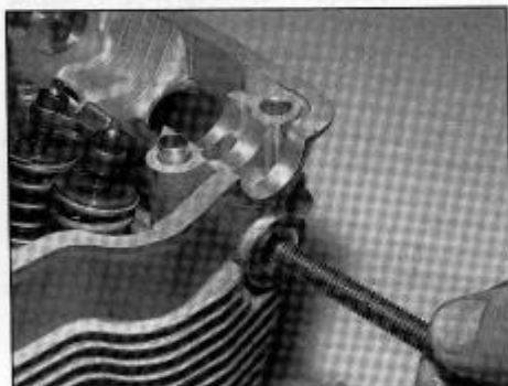
11.35a Thread an M8 bolt into the end of the rocker shaft . . .
