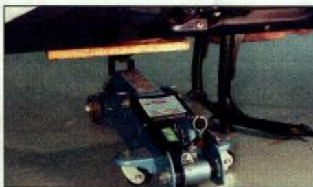
1.4 Always use a block of wood between the engine and jack head when supporting the engine in this way
